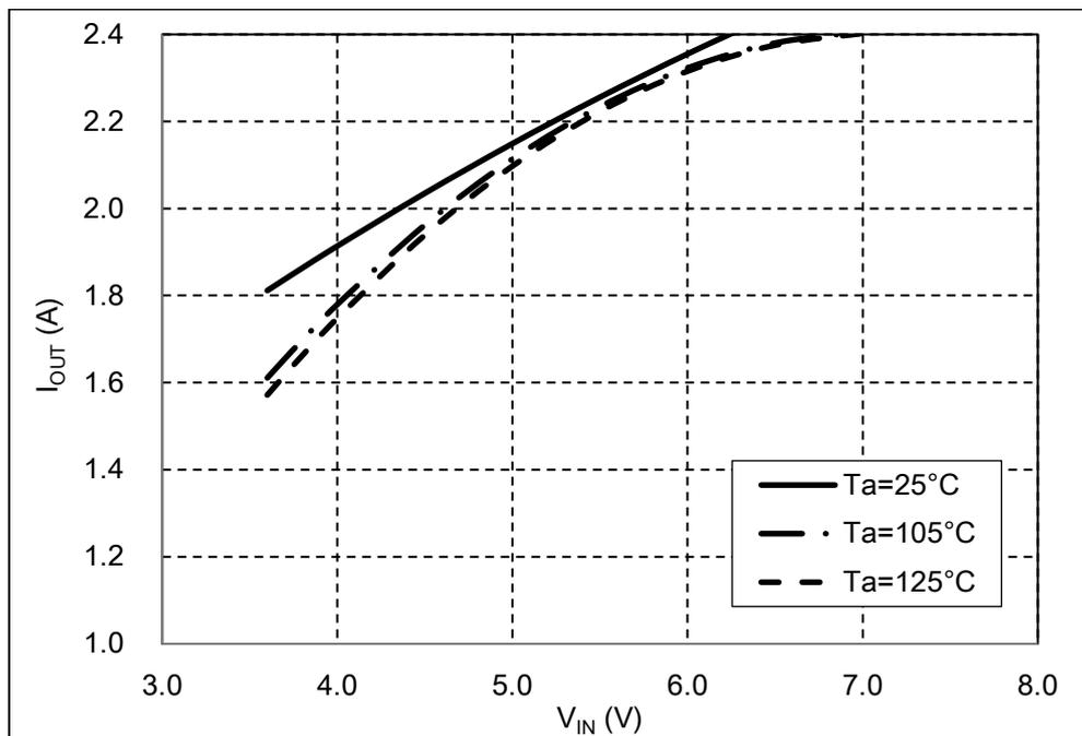
$V_{OUT} = 3.3\text{ V}$  Setting
