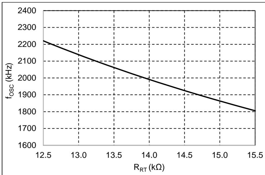
$$R_{RT} \text{ [k}\Omega\text{]} = 37773 \times f_{osc} \text{ [kHz]} ^{-1.04}$$
