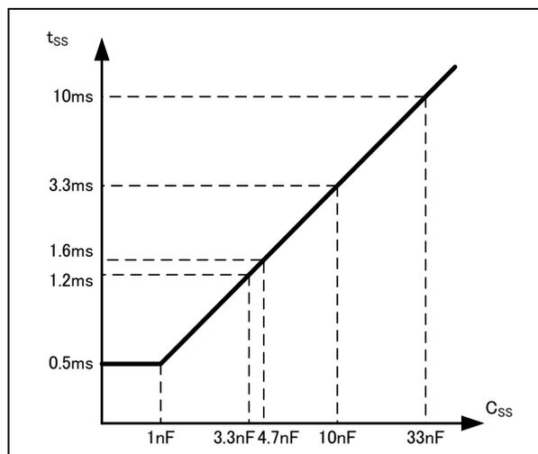
$$C_{SS} [nF] = (t_{SS} - t_{vo\_s}) / 0.64 \times 2.0$$
